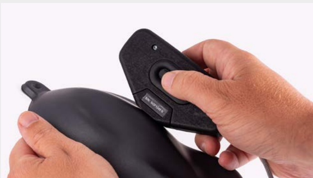
Measures curvature in both directions
